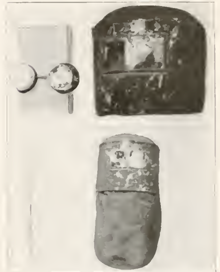
This mask saved both eyes of the workman in an explosion of babbitt metal.
